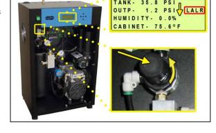
drops **below 2.0 PSI (13.8 KPa) (below 0.30 PSI (2.1 KPa)** – LP Models). After one (1) minute, the Low-Pressure Alarm should appear on the display.
